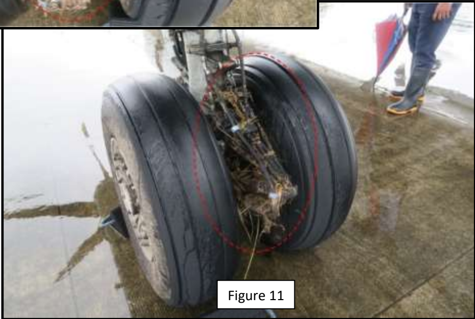
Figure 9-11 – Aircraft landing gears with traces of mud and grass.
