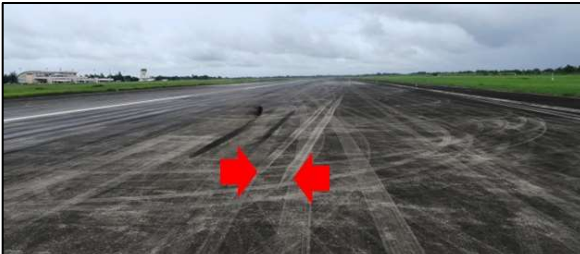
Figure 6 – Tire marks from the aircraft's MLG at the touchdown point.
