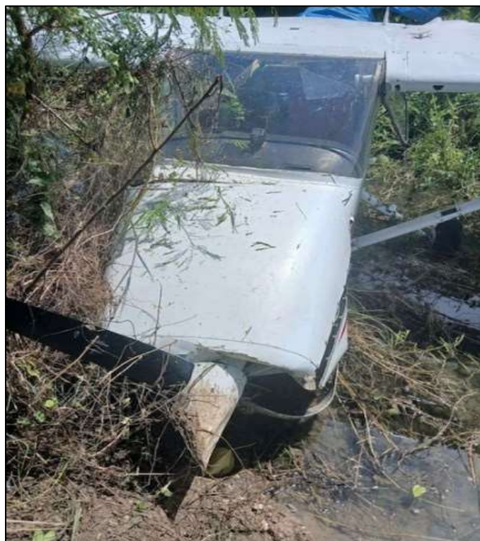
Figure 3 - RP-C7730 impact damage on the propeller.
