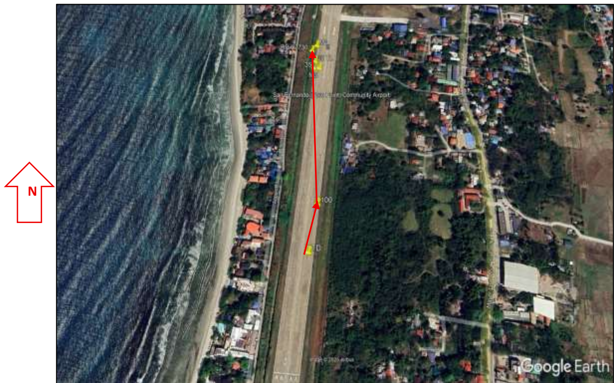
Figure 6 – The aircraft touch down (TD) zone and path going out of the runway.
