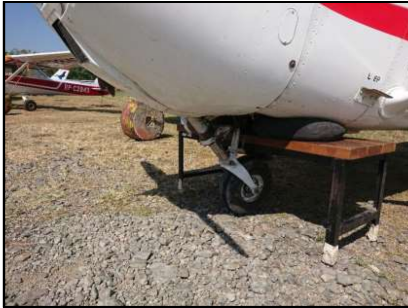
Figure 3. The aircraft nose landing gear assembly was damage upon impact with the fence.
