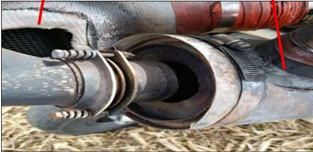
Figure 4 - The Exhaust Shroud Muffler System and Air Induction System assembly.
