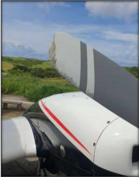
Figure 6 - RP-C 4321 Nicks at left propeller blade.
