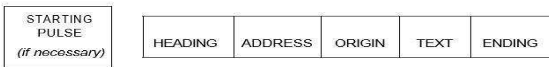
Figure 2.4-2. Form of transmission – teletypewriter operation (see 2.4.4.10.1.2)
