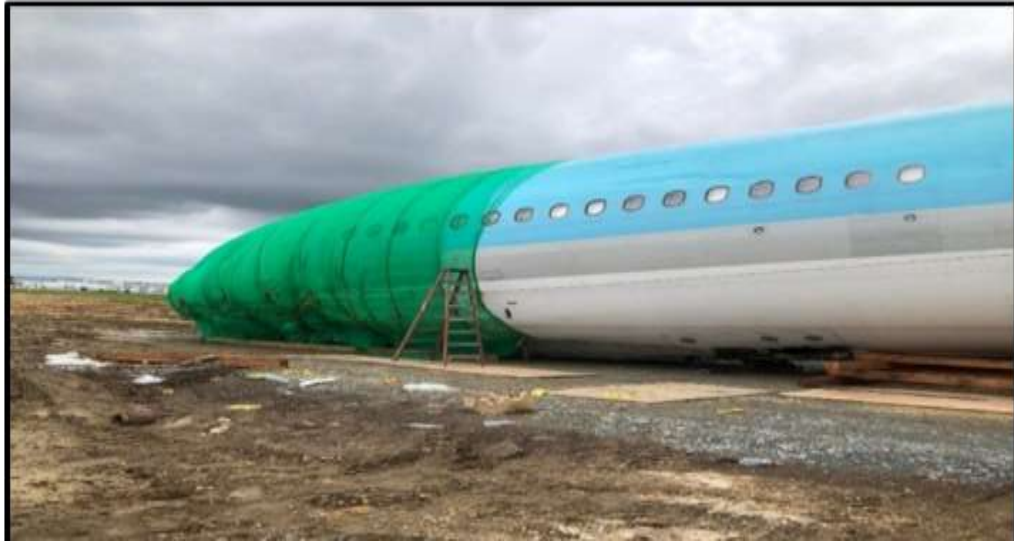
Figure 50 - The aircraft with collapsed NLG at the temporary relocation area.
