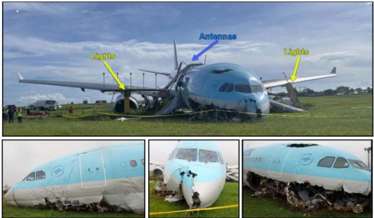
Figure 6 - The aircraft rested on its nose the lower part of the forward fuselage heavily damaged
