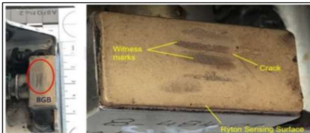
Figure 28 - The witness marks found in the RH MLG (8GB) sensor.
