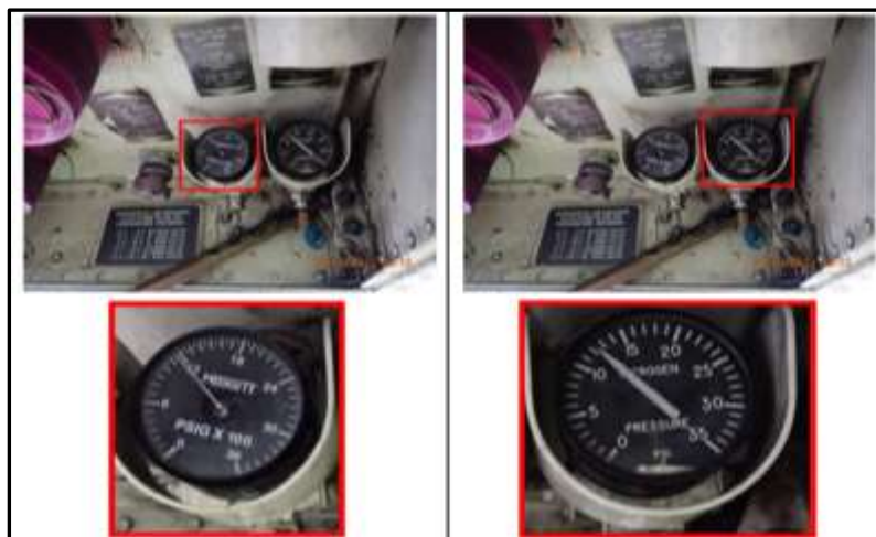
Figure 32 - The aircraft brake pressure accumulator gauges during inspection.
