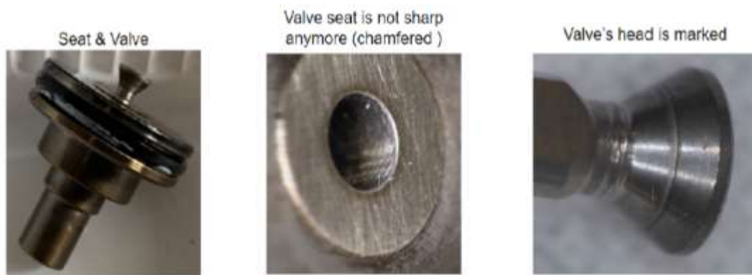
Figure 36 - Damage in the seat and valve
