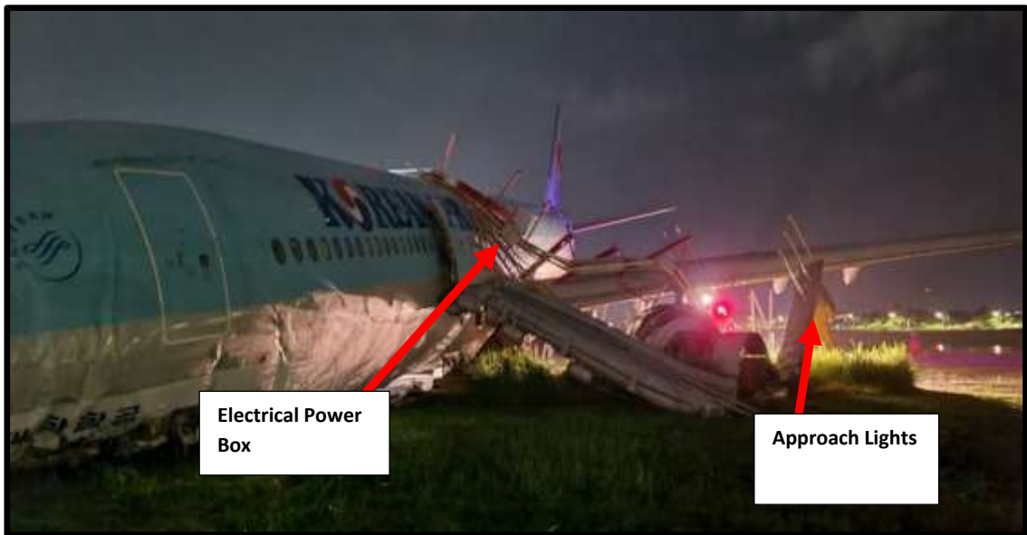
Figure 8 - The aircraft left wing colliding with the Electrical Power box and Approach lights.
