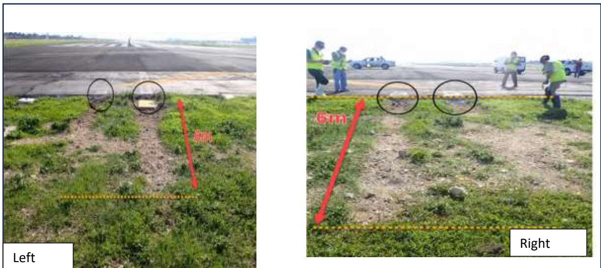
Figure 11 and 12 - The aircraft main landing gear tire marks before the paved portion of RWY 22.
