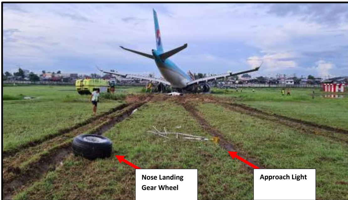
Figure 9 - Presence of the detached NLG wheel was observed within the path of the aircraft.
