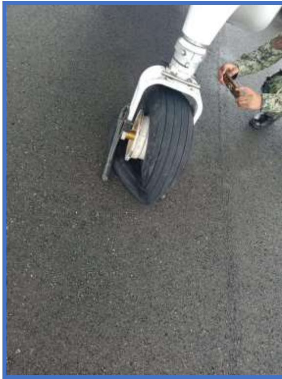
Figure 3: Deflated nose gear strut and tire
