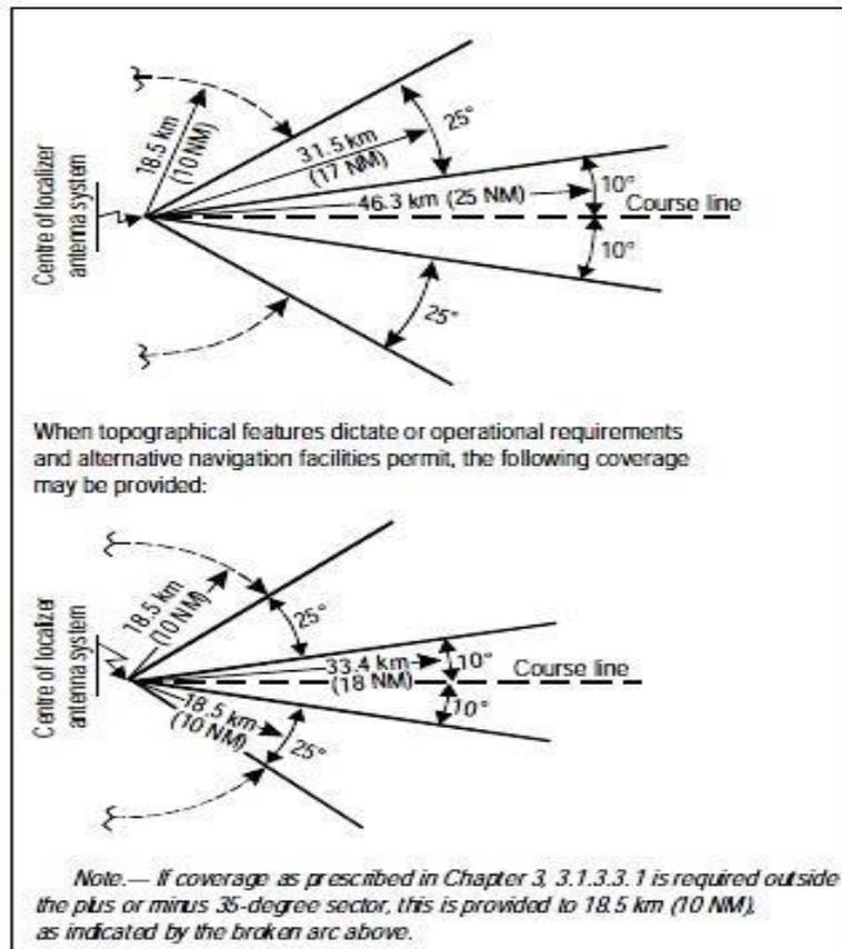
Figure C-7. Localizer coverage with respect to azimuth
