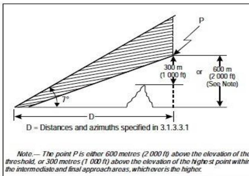
Figure C-8. Localizer coverage with respect to elevation
