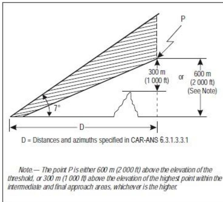
**Figure C-8A. Localizer coverage with respect to elevation**
