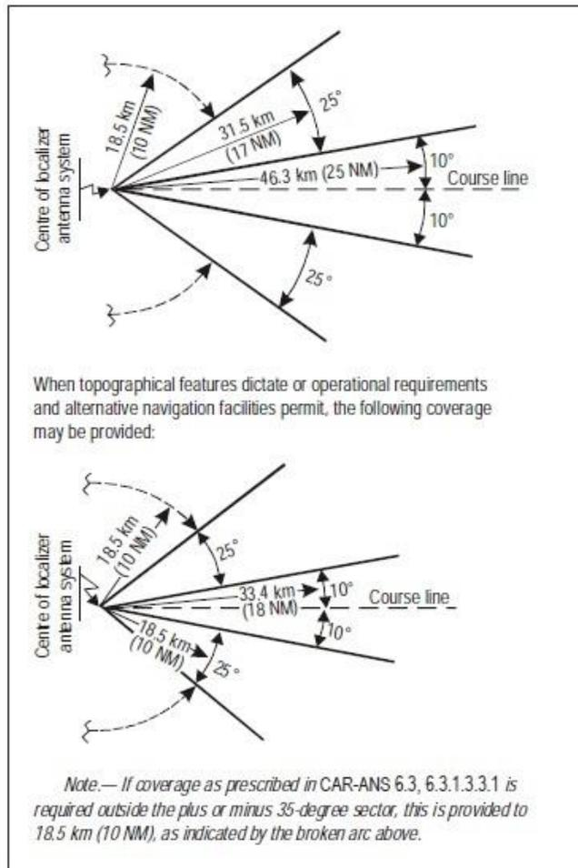
**Figure C-7A. Localizer coverage with respect to azimuth**
