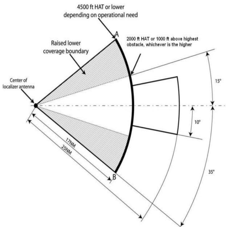
**Figure C-7B. Reduced localizer coverage with respect to azimuth**
