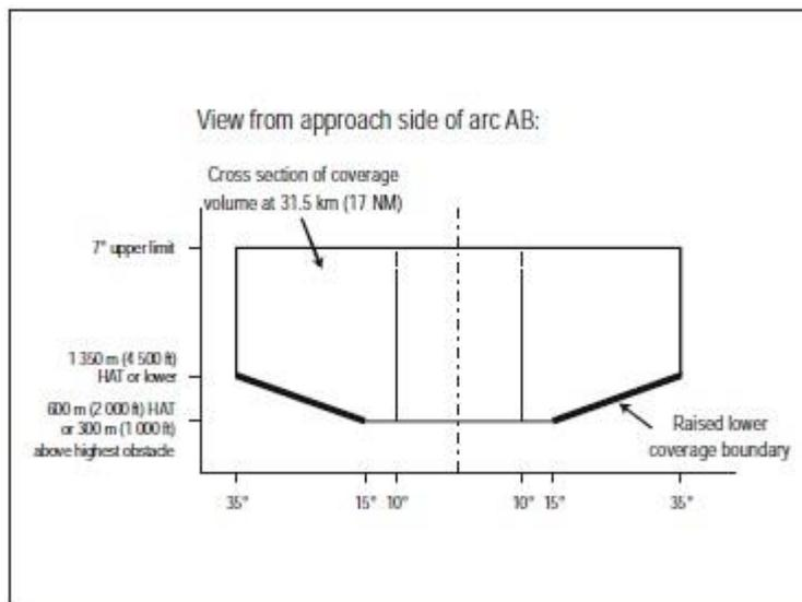
**Figure C-8B. Reduced localizer coverage with respect to elevation**
